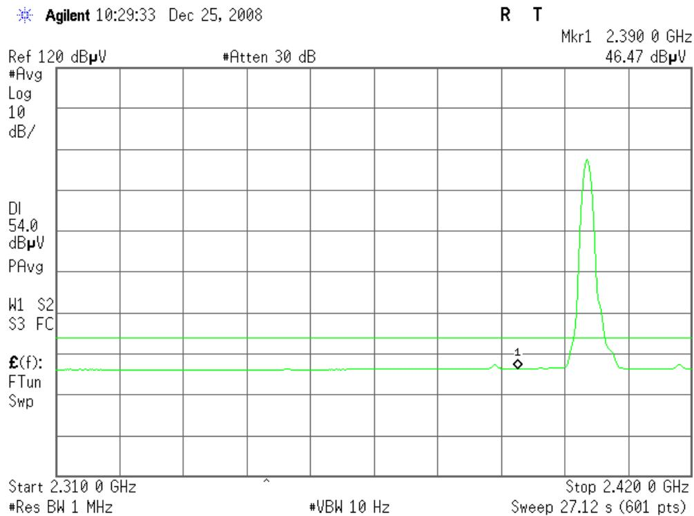
**Band Edges (CH-High)****Detector mode: Peak****Polarity: Vertical**
