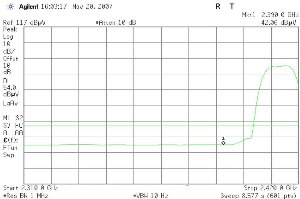
**Band Edges (IEEE 802.11b / CH High)****Detector mode: Peak****Polarity: Vertical**
