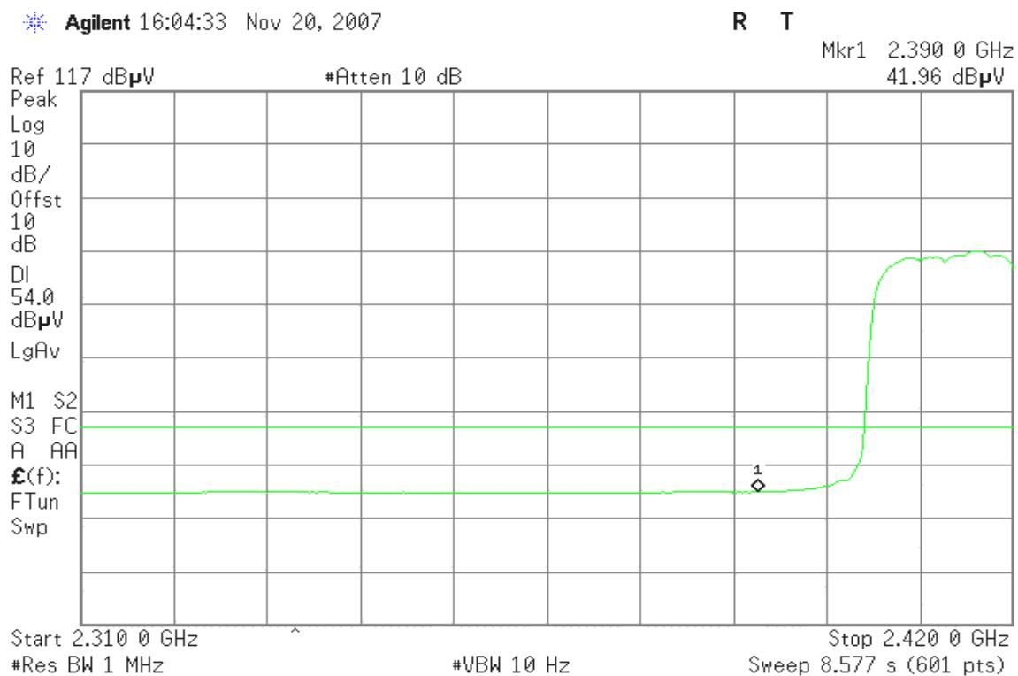
**Band Edges (IEEE 802.11g / CH High)****Detector mode: Peak****Polarity: Vertical**
