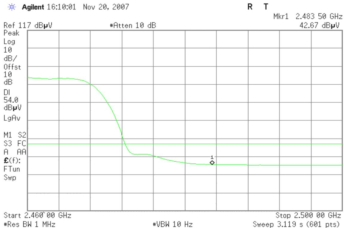
**Band Edges (IEEE 802.11g / CH Low)****Detector mode: Peak****Polarity: Vertical**
