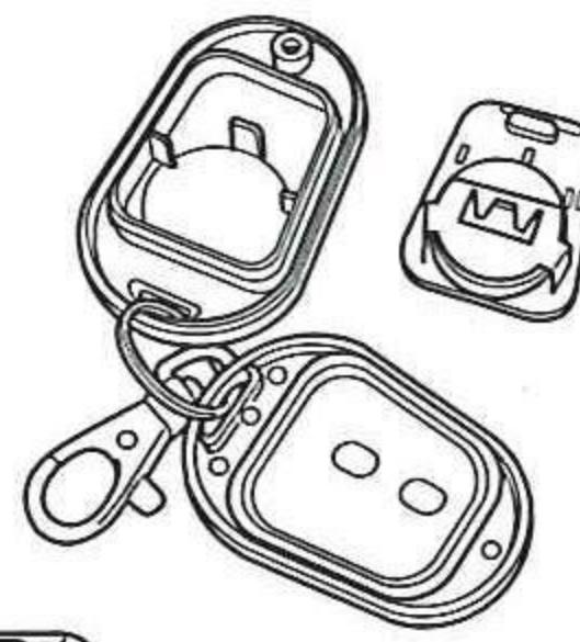
2. Take out the dry cell batteries in the direction of (a).
