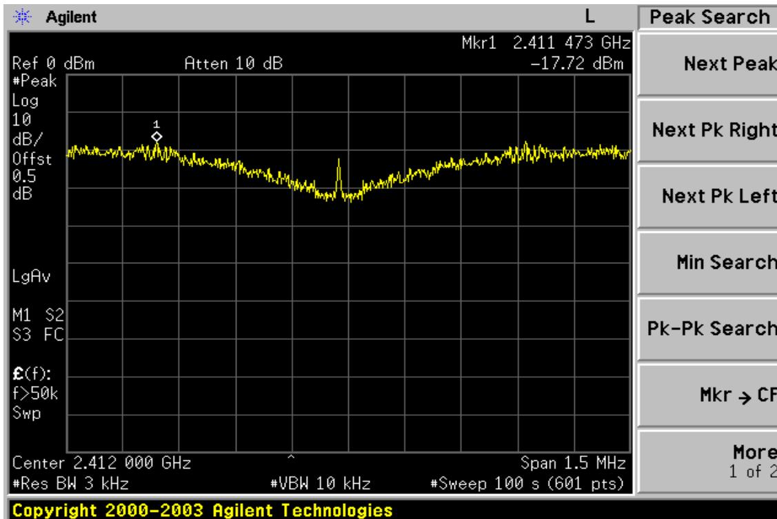
**Power Spectral Density Test Plot (CH-Mid)**
