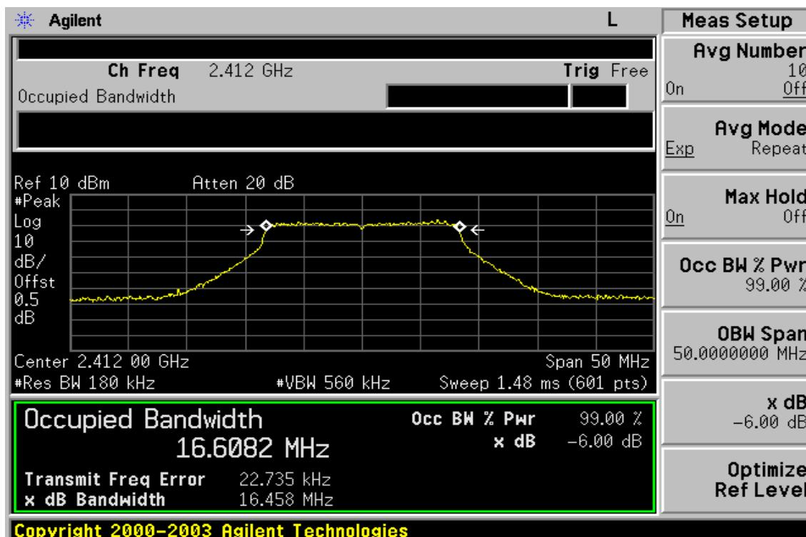
**Copyright 2000-2003 Agilent Technologies****6dB Band Width Test Data CH-Mid**
