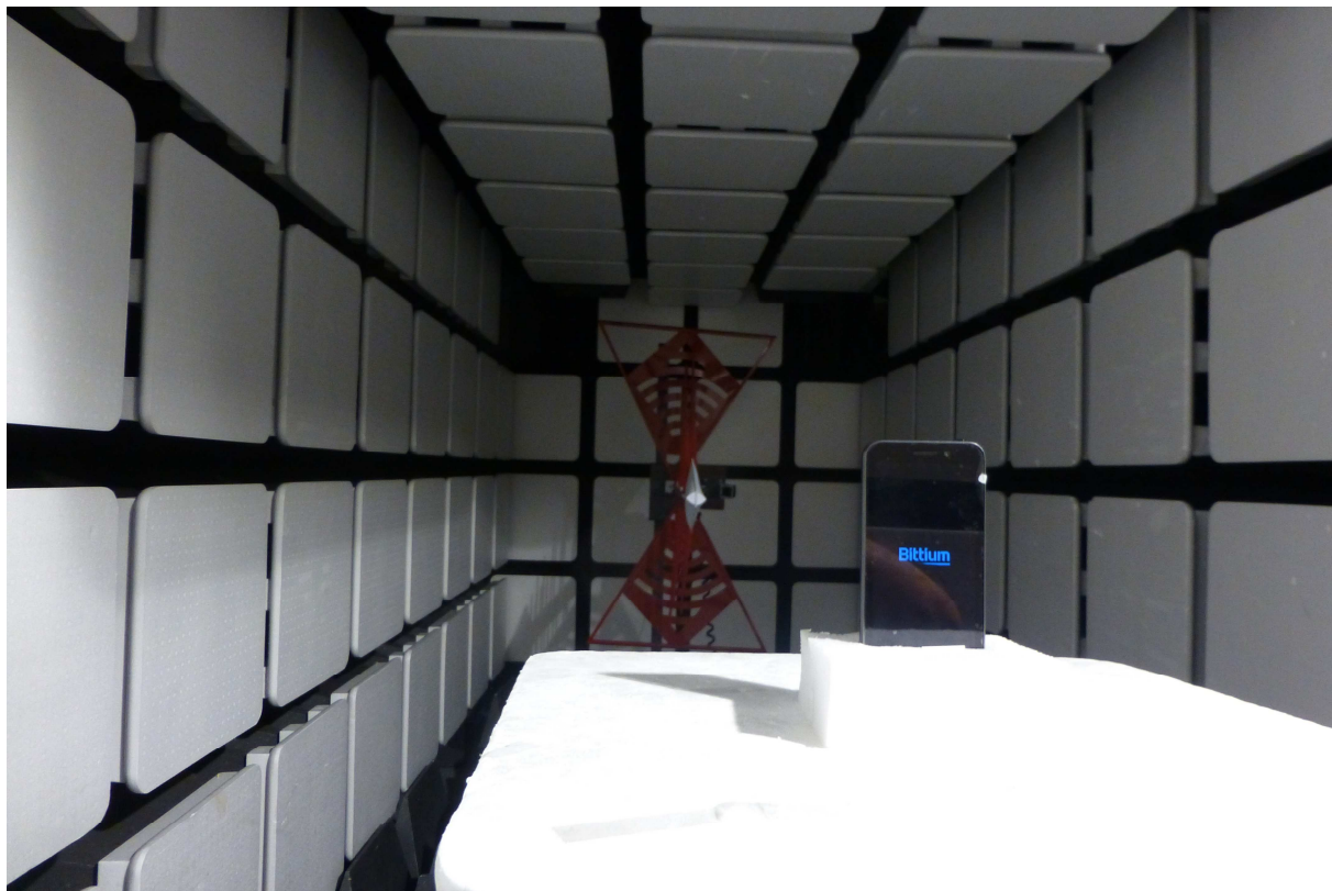
Radiated test setup 30 – 1000 MHz, EUT vertical
