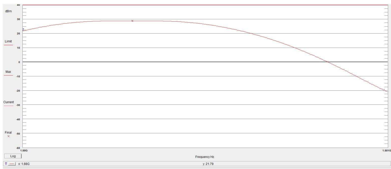
Picture 24: GSM 1900, Ch. 661, RF power output, RBW 300kHz, VBW 300 kHz
