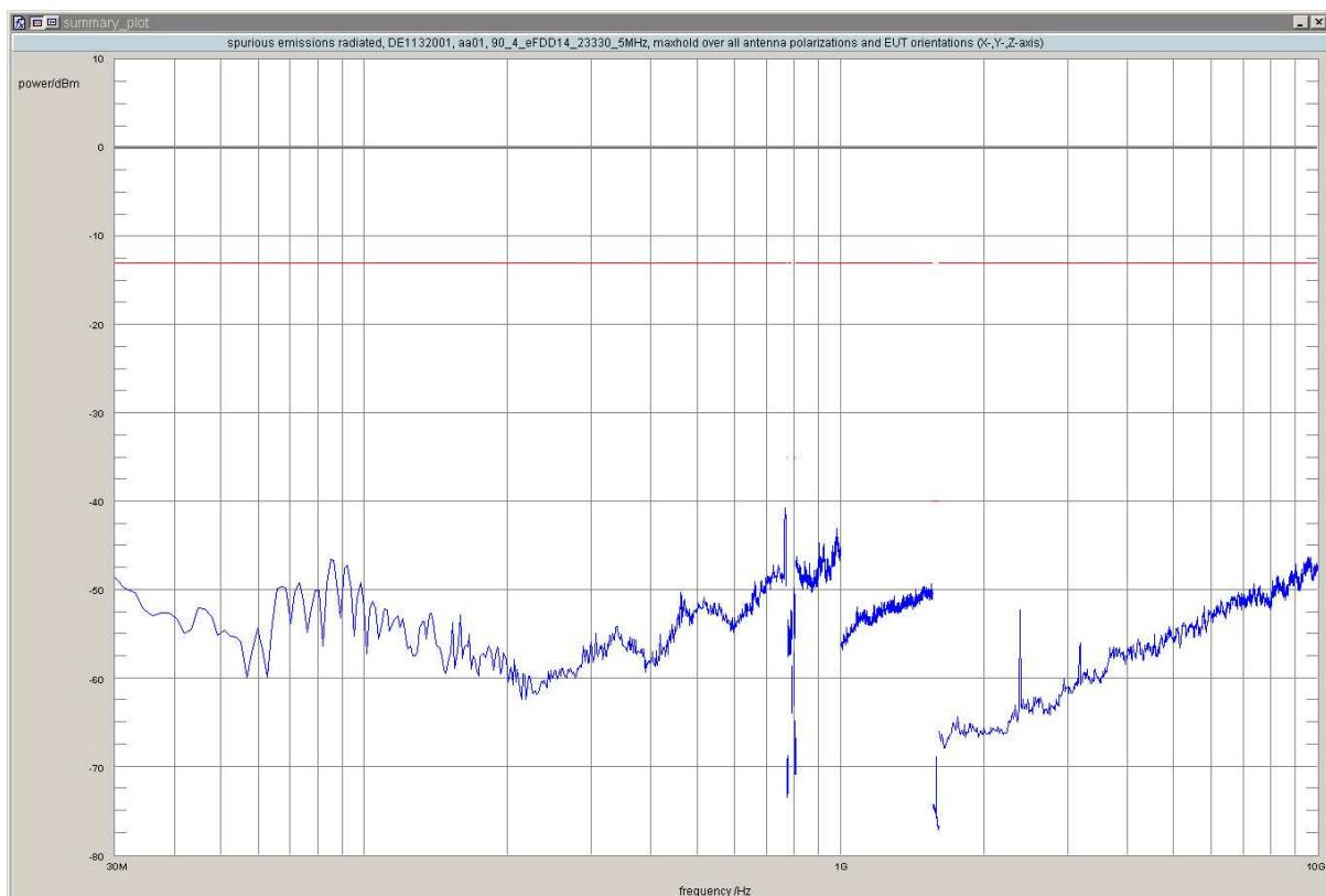
**Test: 90.5; Frequency Band = eFDD14, Mode = QPSK 5MHz, Channel = 23355, Frequency = 795.5MHz, Method = radiated**
