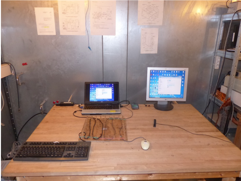
Photo 6: Test setup for conducted measurements (computer peripheral setup, EUT supplied by USB-cable from computer, charging mode, unintentional radiator §15)
