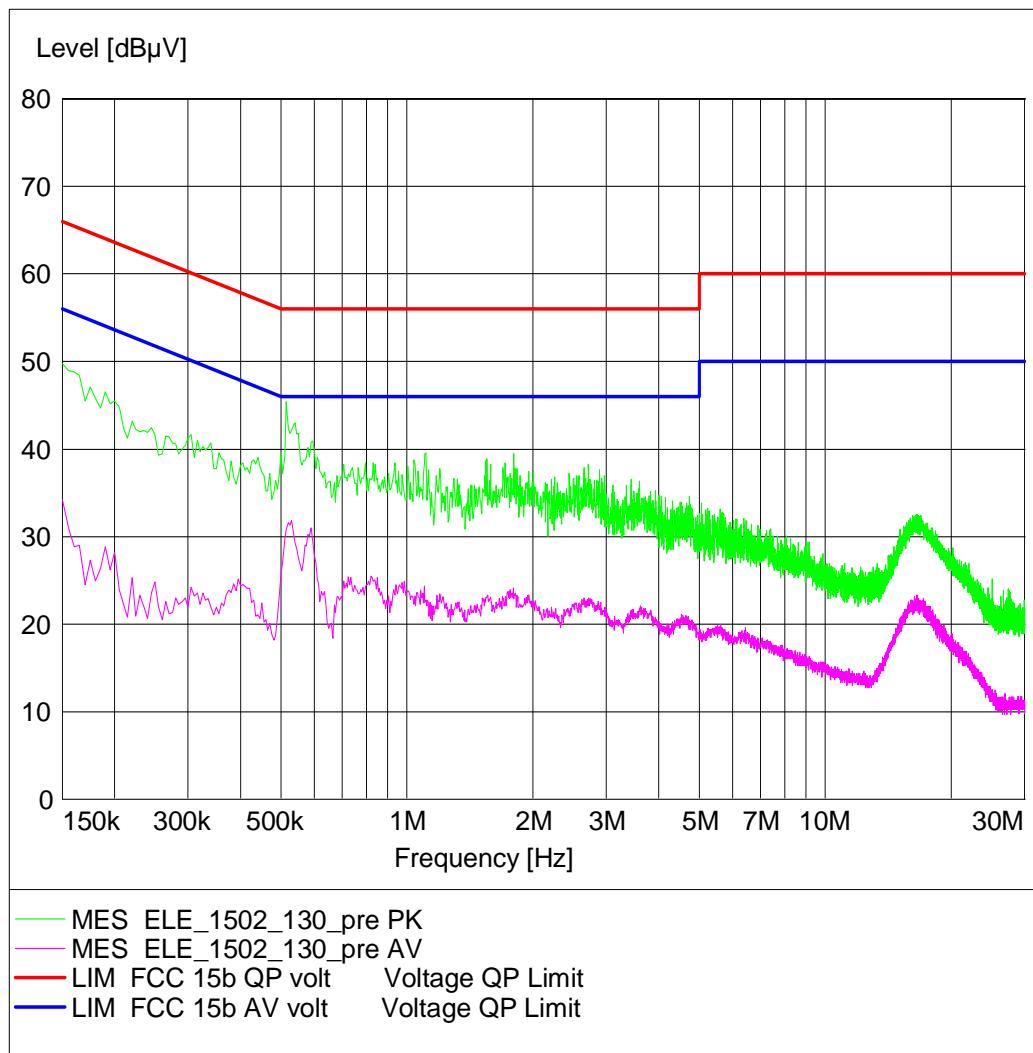
**Test1: 15b.1; Mode = Generating a high power consumption**
