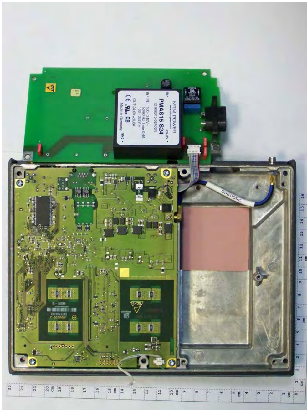
Photograph 5: Overall top view of equipment with main and power PCB
