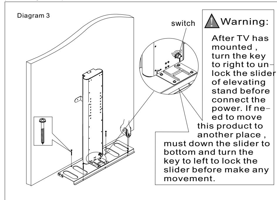
4. Connect the power supply and turn on the switch, use remote control or manual control to rise the elevating stand to the top position, then fix the wall mounting rack to the wall by ⑨expansion screws, and connect the base plate and elevating stand by ⑧M6X10mm screws. (see diagram 4)
