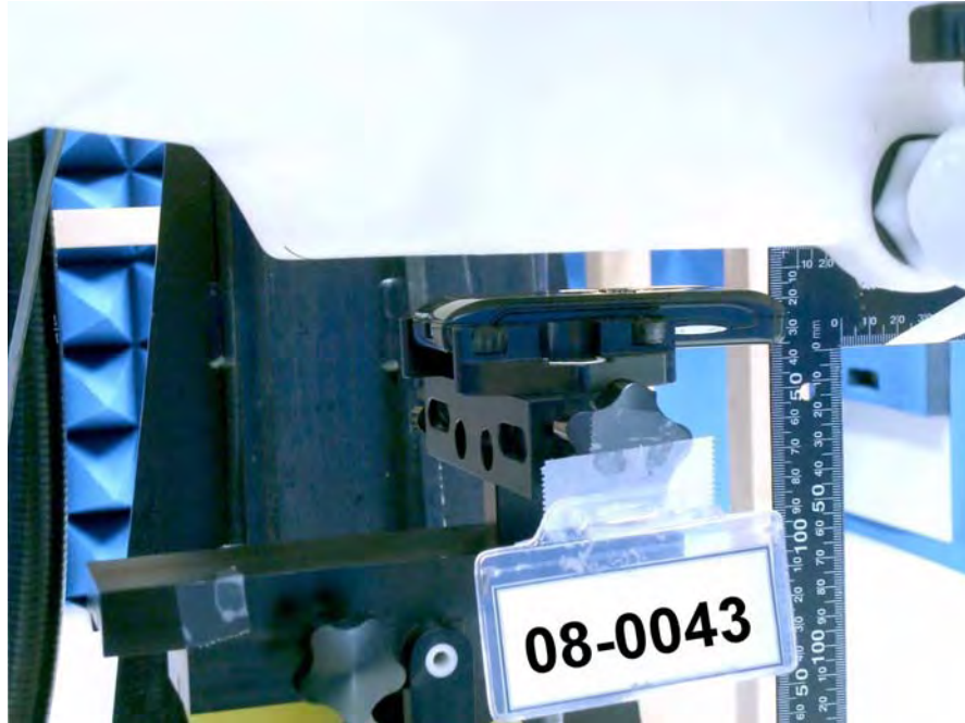
Figure 13.Body SAR Test Setup (Flat Section) _ 15 mm separation
