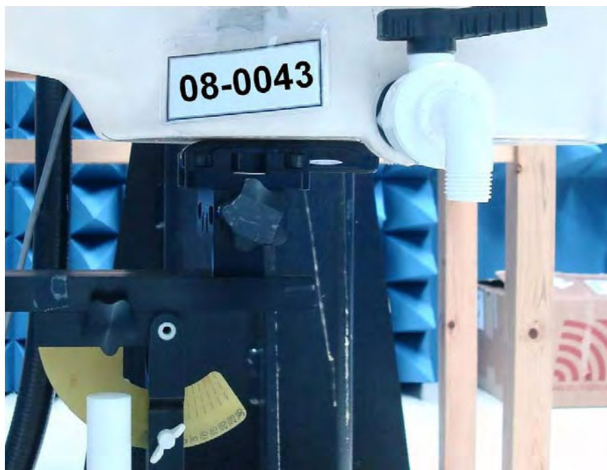
Figure 14.Body SAR Test Setup (Flat Section) _ 0 mm separation
