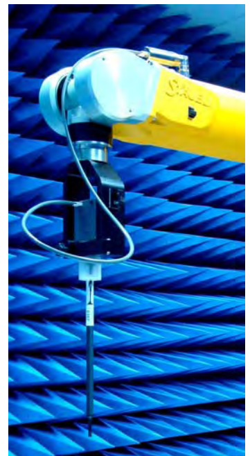
Figure 5. Probe setup on robot
