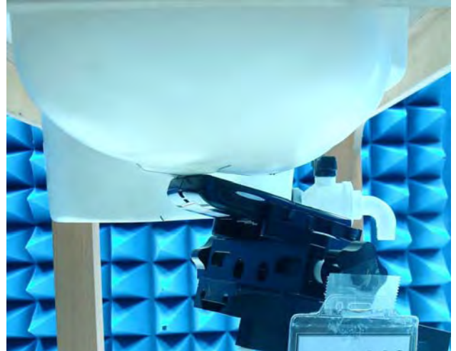
Figure 20. Right Head SAR Test Setup (Tilted)
