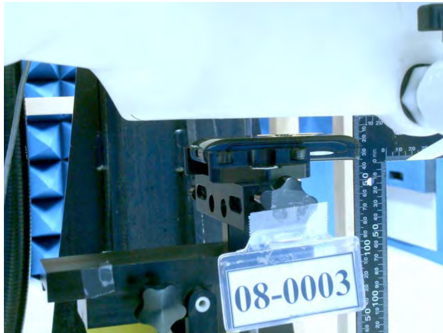
Figure 23.Body SAR Test Setup (Flat Section) _ 15 mm separation
