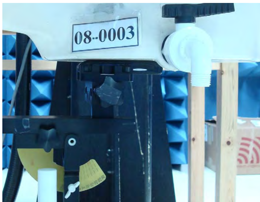
Figure 24.Body SAR Test Setup (Flat Section) _ 0 mm separation
