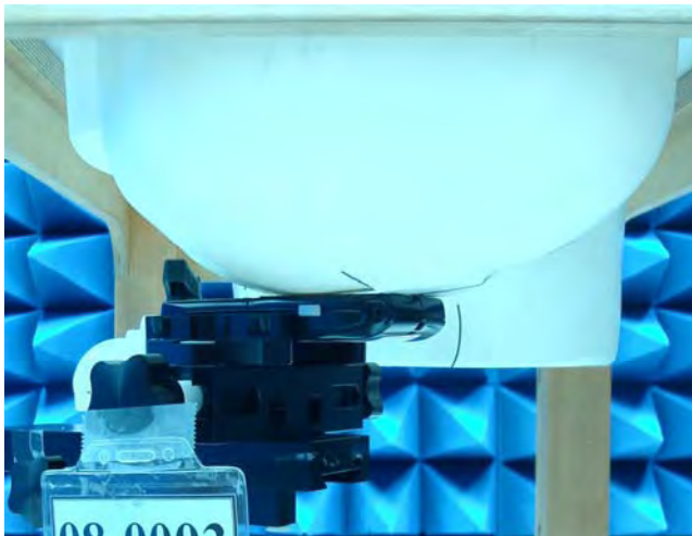
Figure 21. Left Head SAR Test Setup (Cheek)
