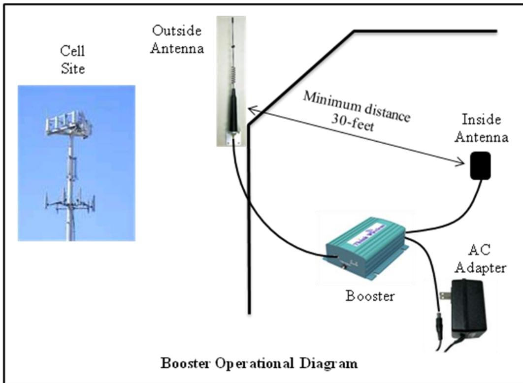
The TWDBMPSB-01 system contains a dual band low power indoor antenna, amplifier/repeater unit and high gain omni-directional outdoor antenna. The outdoor omni-directional antenna must be installed and operate in a vertical position.
