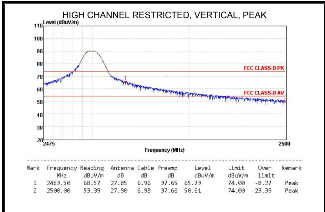
Note: EUT in each of three orthogonal axis emissions had been tested, but only the worst case
