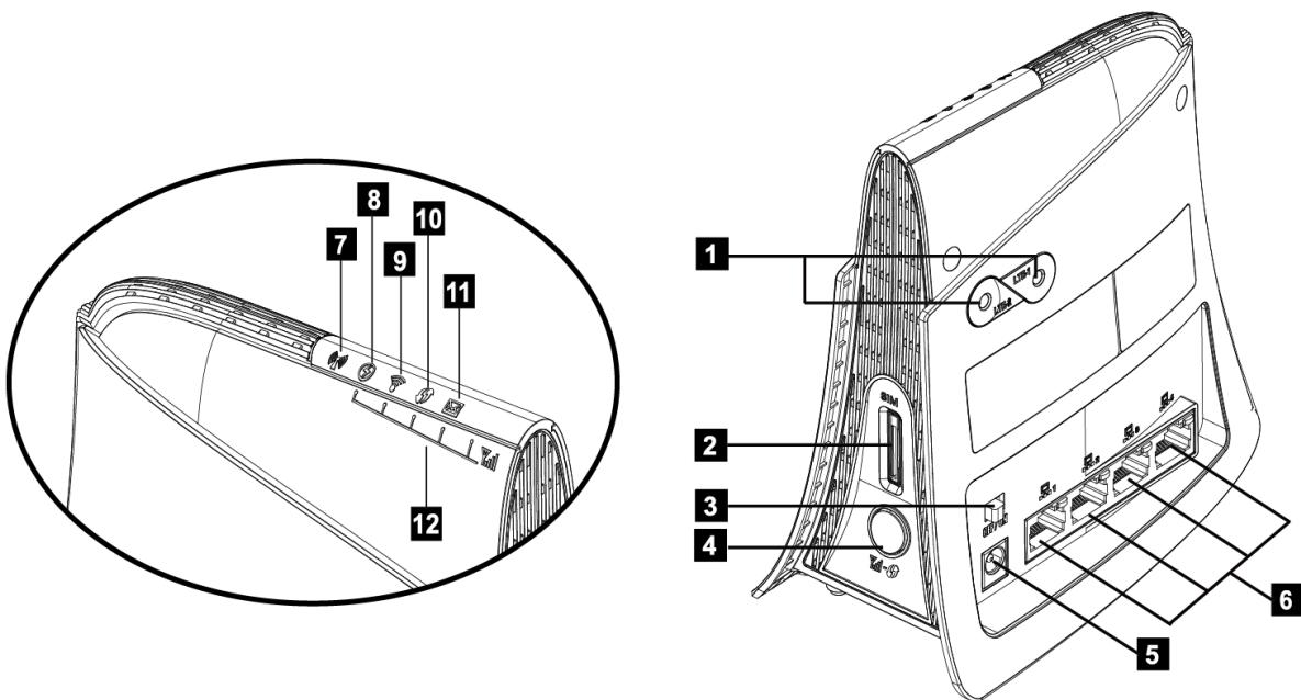
**1 4G External Antenna Ports** Connect 4G External Antennas if needed.
