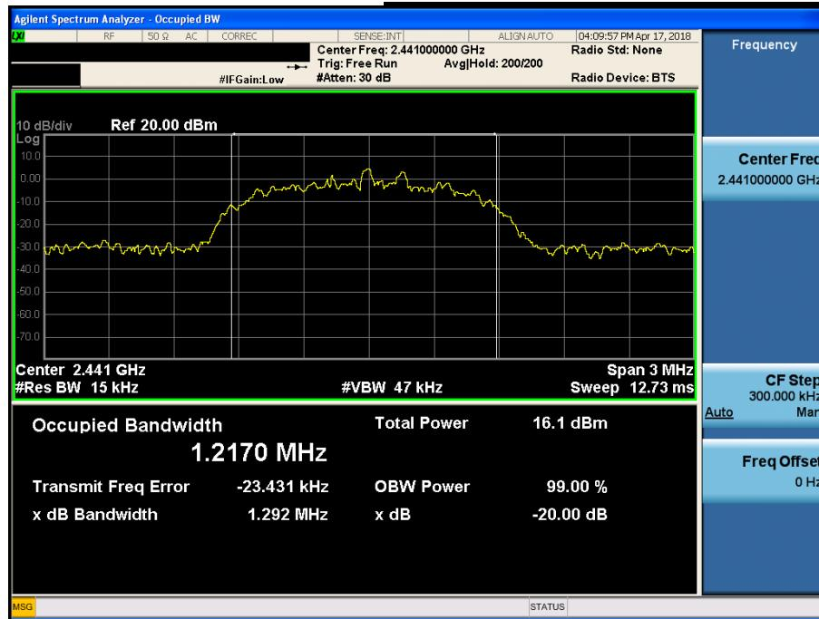
**20 dB Bandwidth****Highest Channel & Modulation : 8DPSK**
