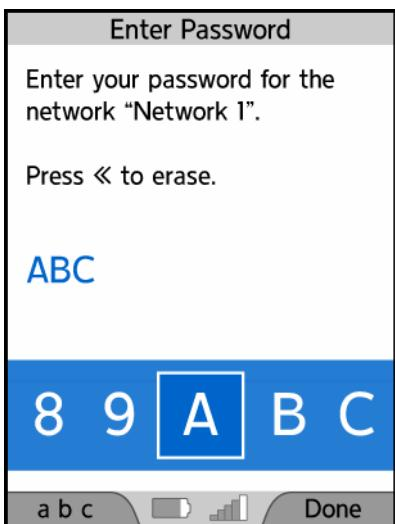
If the network requires a password, the Enter Password screen will appear. To start entering the password, turn the thumbwheel to highlight the first character, and press SELECT. If you need to change from uppercase letters to lowercase, or to find a special character, press the LEFT button. Continue selecting letters until the password is complete, and press the RIGHT button.
