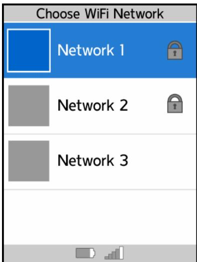
When starting the WiFi connection, your Sansa Connect will find all of the WiFi networks in range. Networks will be listed in order of signal strength (highest first), and protected networks (which require a password) are indicated by the lock icon.
