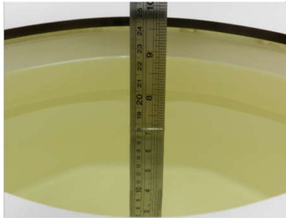
Fig 11.1 Photo of Liquid Height for Body SAR
