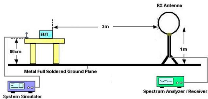
For radiated emissions from 30MHz to 1GHz
