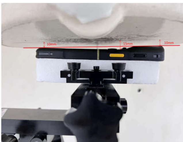
Back _ BLE Beacon, Test Separation 10 mm
