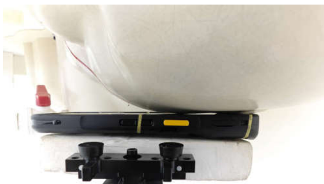
Left Cheek_ BLE Beacon, Test Separation 0 mm
