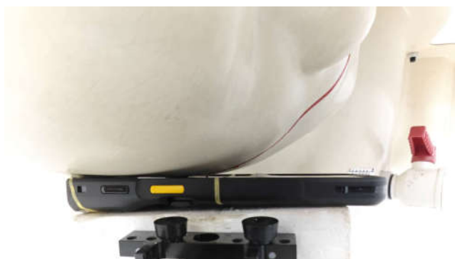
Right Cheek_ BLE Beacon, Test Separation 0 mm
