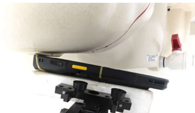
Right Tilted _ Extended, Test Separation 0 mm
