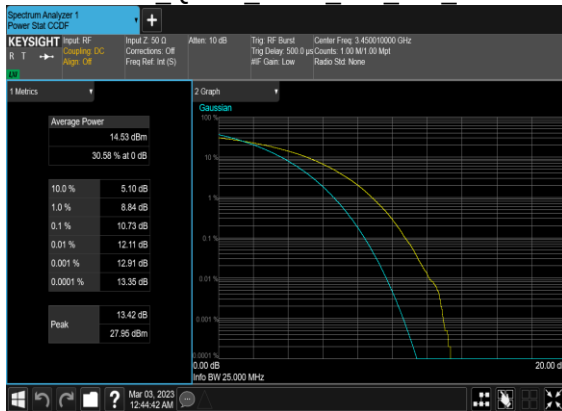
N77(100M)_CP- OFDM QPSK Outer Full Mid CH
