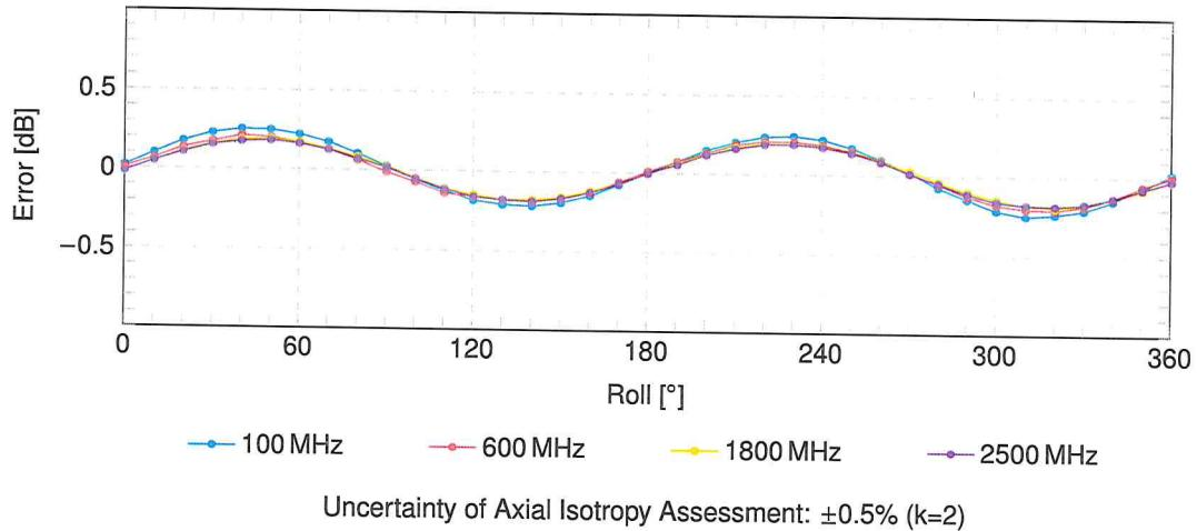
**Receiving Pattern ( $\phi$ ),  $\vartheta = 90^\circ$**
