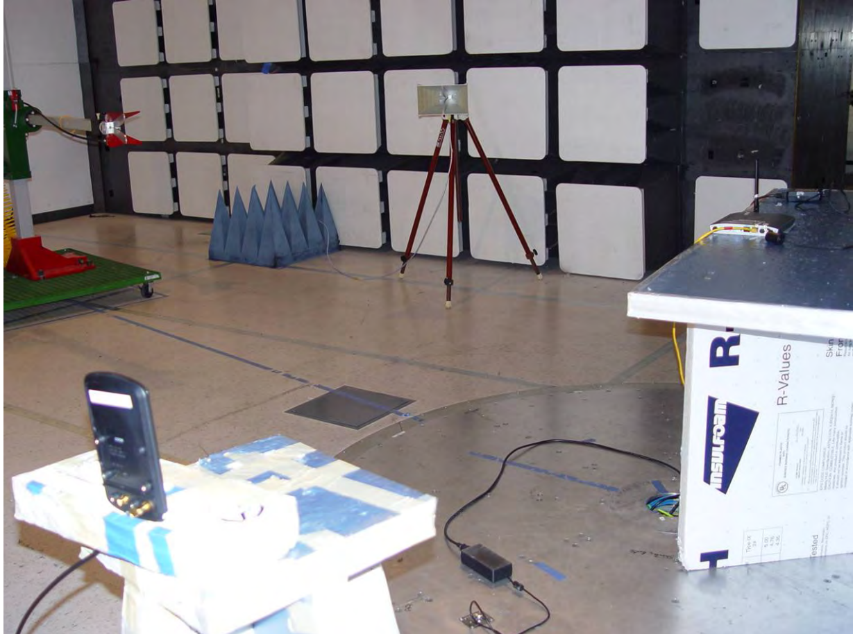
General Radiated DFS Test Setup
