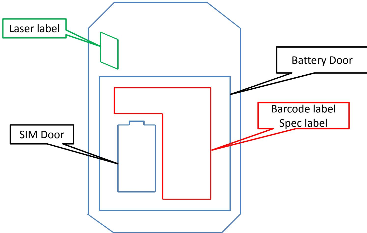
Label located in the battery compartment and is visible to the users as they install the SIM card.
