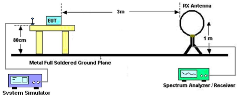
For radiated test from 30MHz to 1GHz
