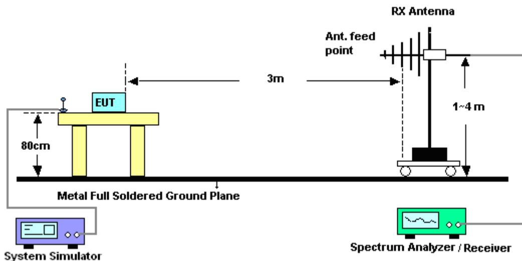
For radiated test above 1GHz
