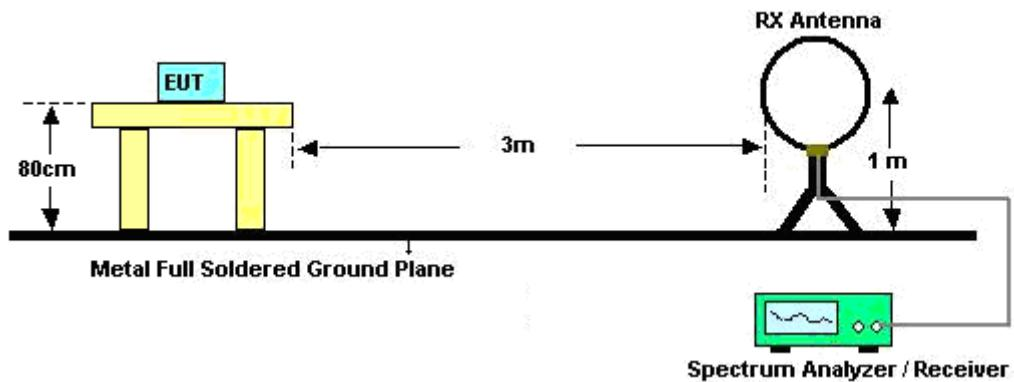
For radiated emissions from 30MHz to 1GHz
