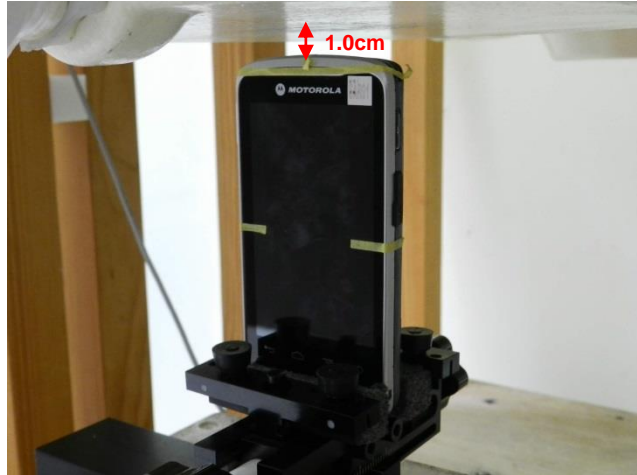
Top Side With Battery 1,Test Separation 1 cm
