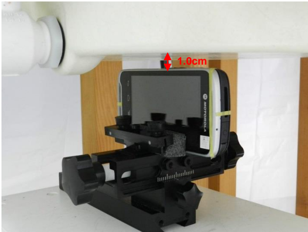
Left Side With Battery 1,Test Separation 1 cm
