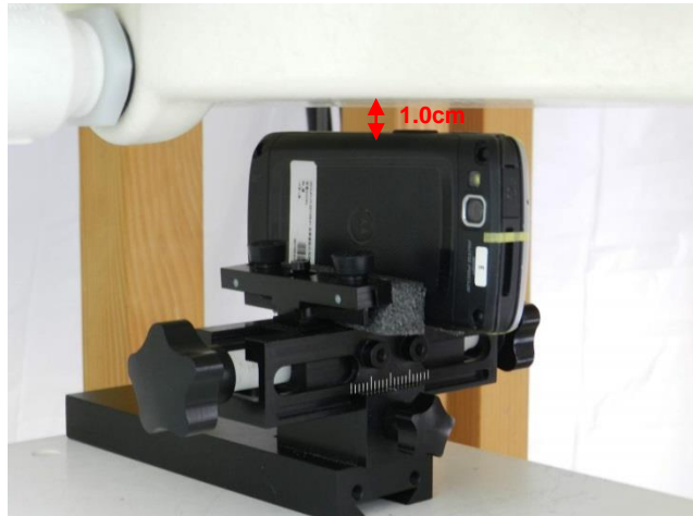
Right Side With Battery 1,Test Separation 1 cm
