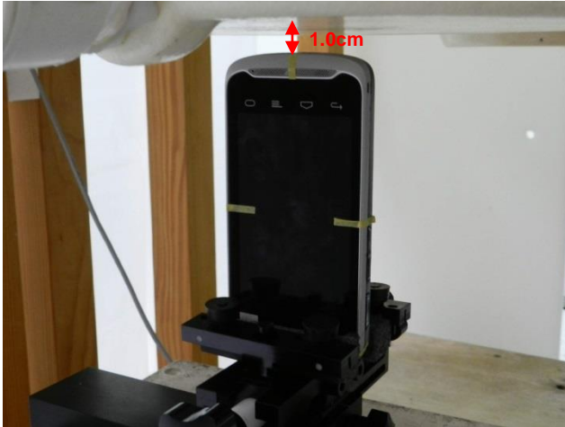
Bottom Side With Battery 1,Test Separation 1 cm
