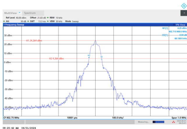
20 dB Bandwidth Plot on 927.25 MHz
