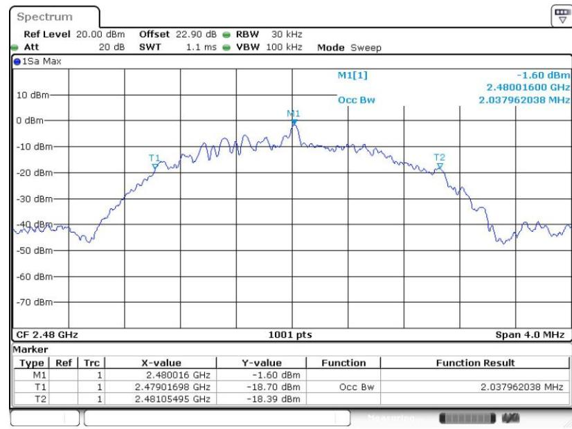
Note: The occupied channel bandwidth is maintained within the band of operation for all of the modulations.
