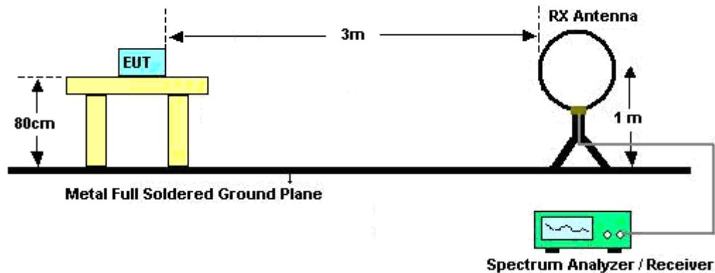
For radiated emissions from 30MHz to 1GHz
