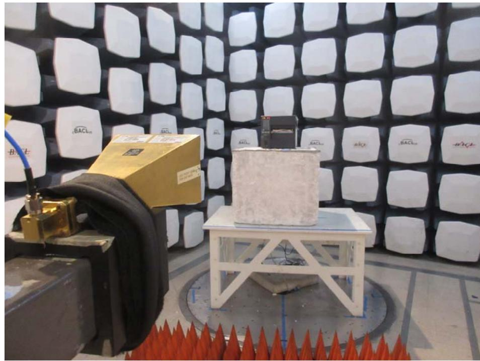
**1.12 Radiated Spurious Emissions: 18 GHz to 26.5 GHz, Rear View at 3 meters distance**
