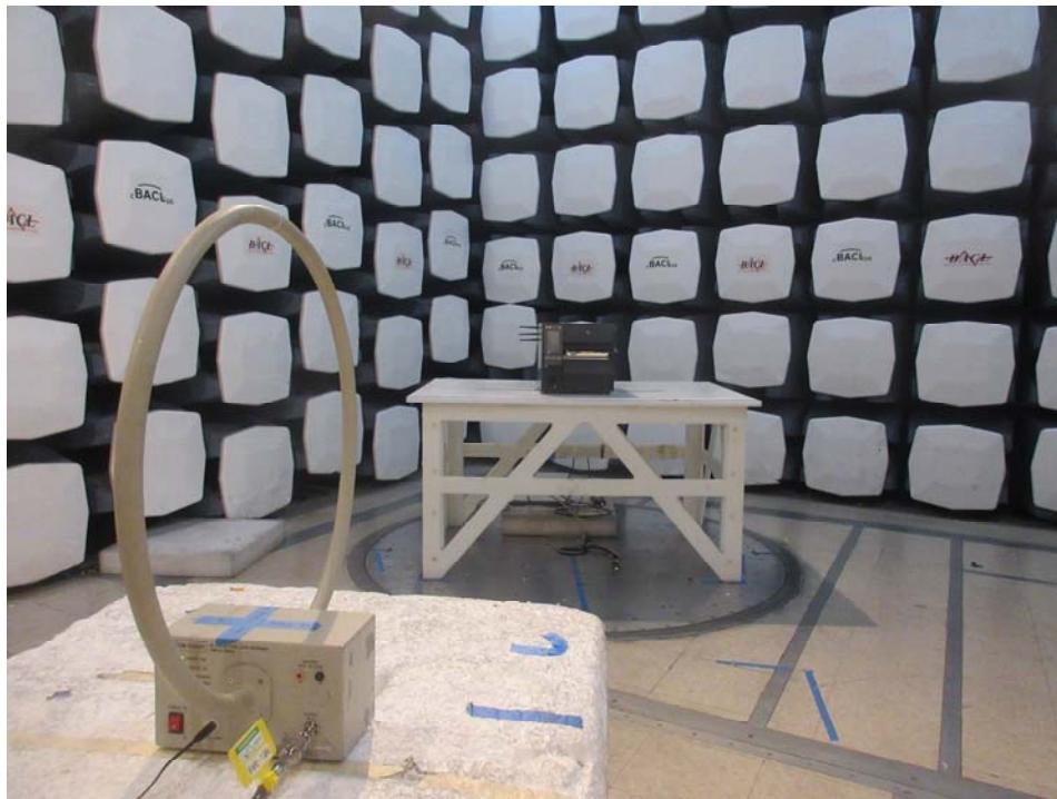
**1.4 Radiated Spurious Emissions: 9 kHz to 30 MHz, Parallel Rear View at 3 meters distance**
