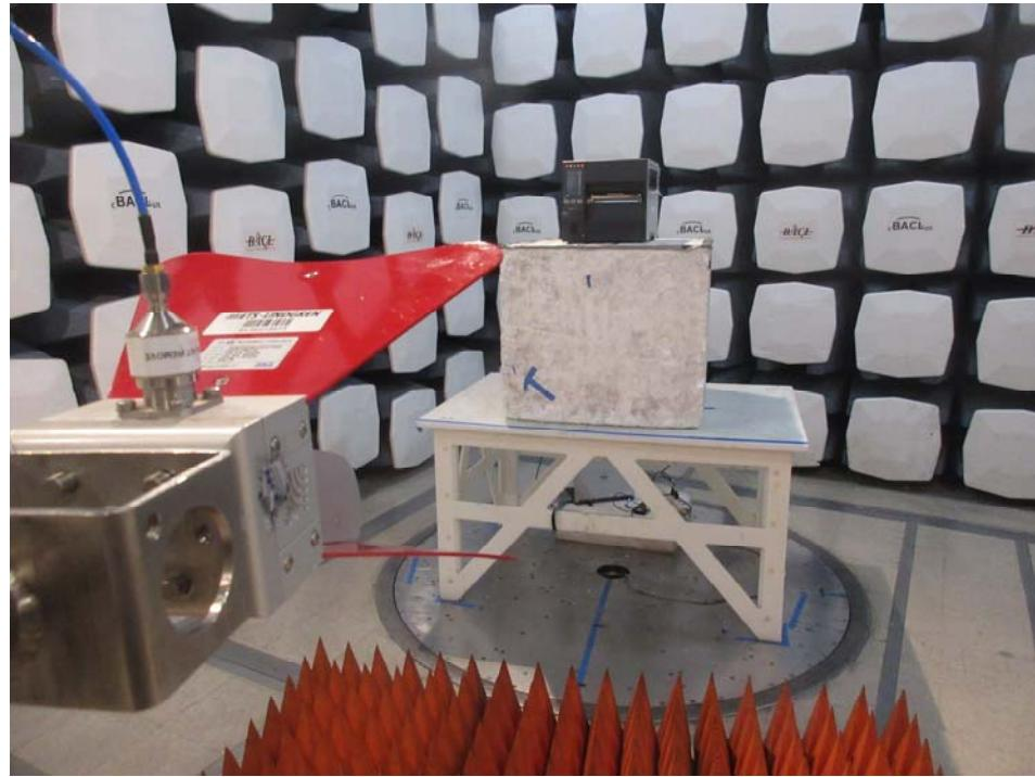
**1.10 Radiated Spurious Emissions: 1 GHz to 18 GHz, Rear View at 3 meters distance**
