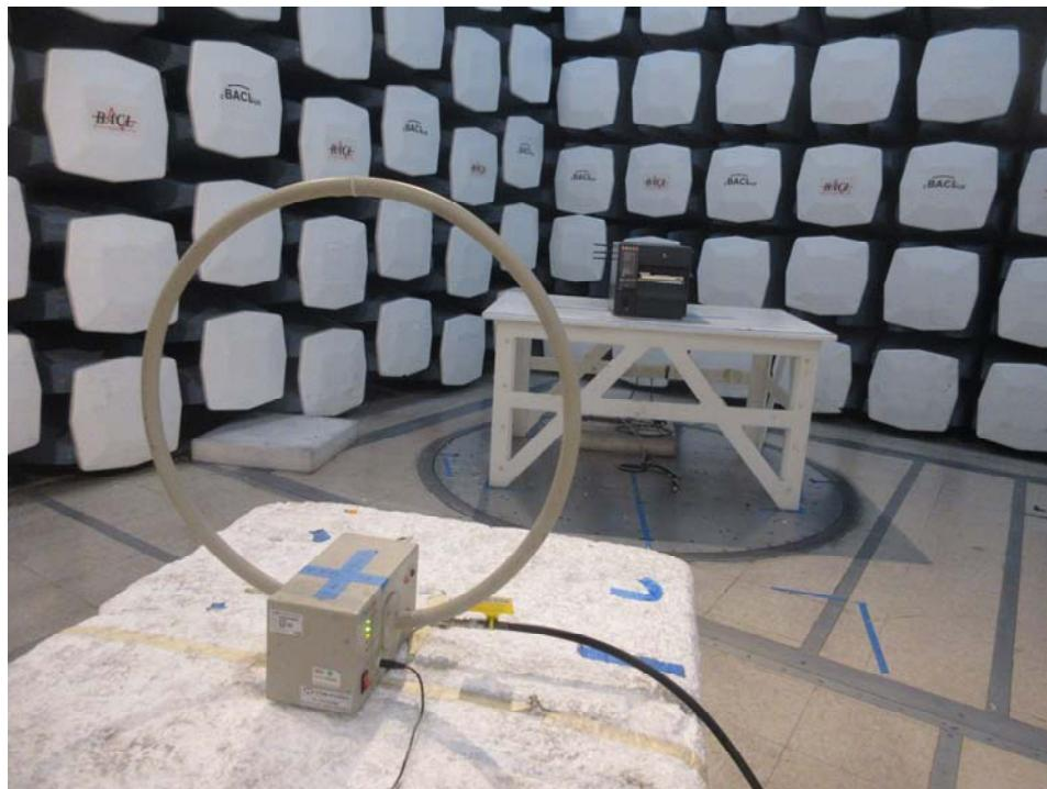
**1.6 Radiated Spurious Emissions: 9 kHz to 30 MHz, Perpendicular Rear View at 3 meters distance**
