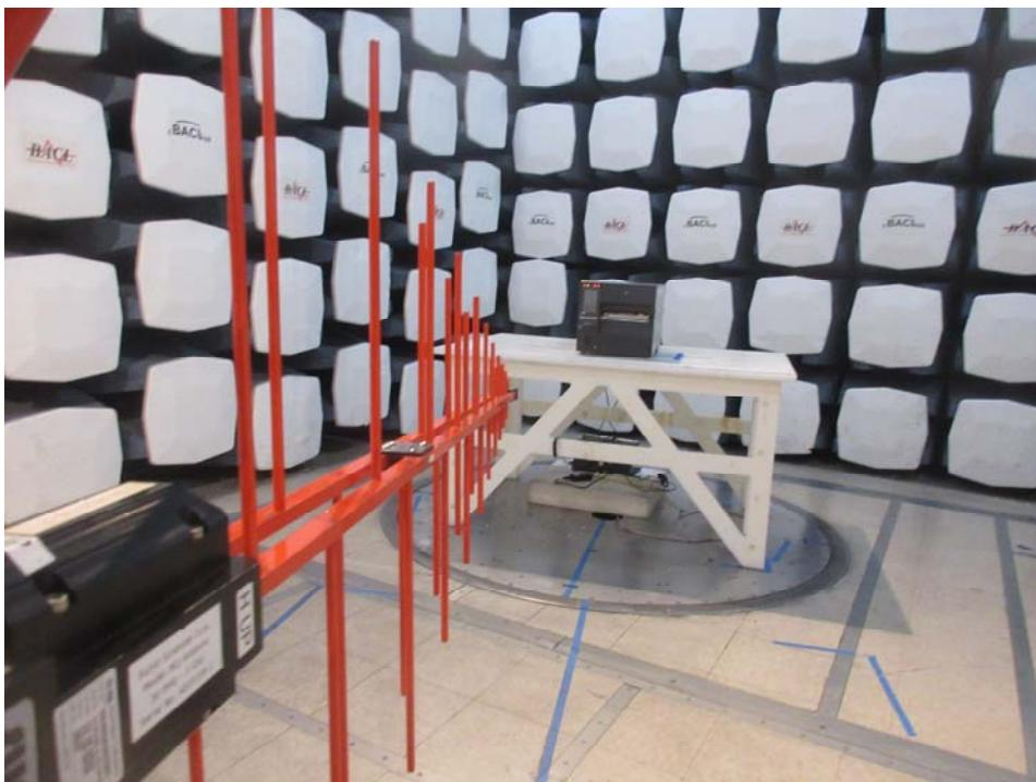
**1.8 Radiated Spurious Emissions: 30 MHz to 1000 MHz, Rear View at 3 meters distance**
