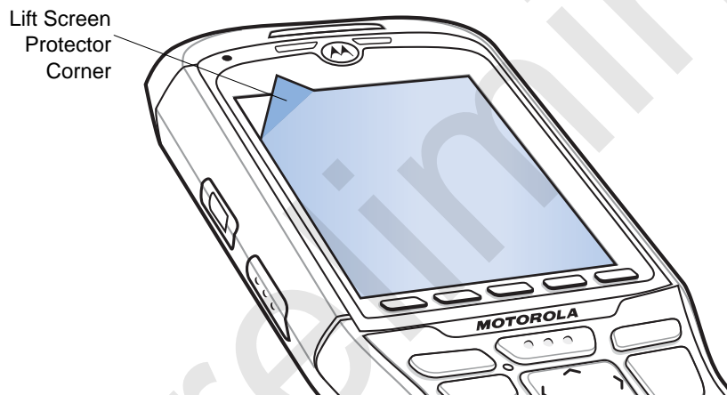
Figure 9-1 Removing the Screen Protector
