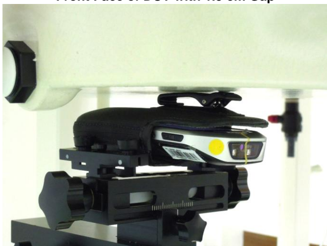
Front Face of EUT, and Holster with 0 cm Gap
