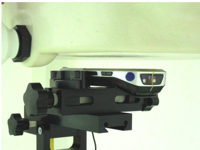
Front Face of DUT with 1.5 cm Gap
