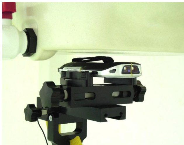
Rear Face of DUT with 1.5 cm Gap
