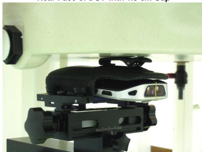
Rear Face of EUT, and Holster with 0 cm Gap
