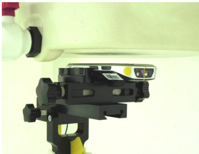
Front Face of DUT with 1.5 cm Gap
