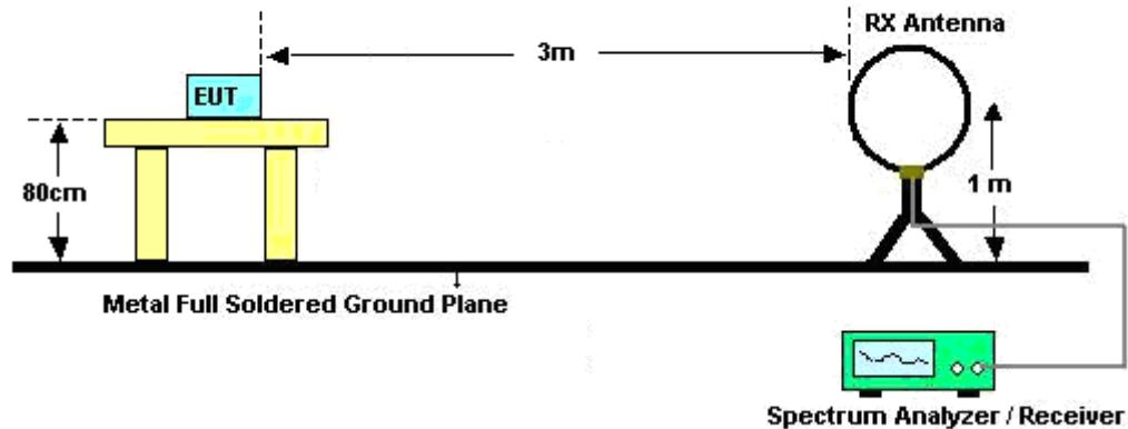
For radiated emissions from 30MHz to 1GHz
