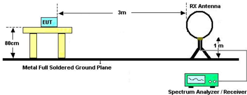
For radiated emissions from 30MHz to 1GHz
