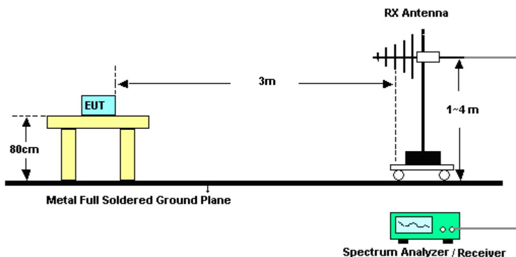
**For radiated emissions above 1GHz**
