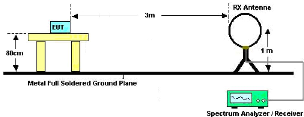
For radiated emissions from 30MHz to 1GHz
