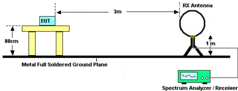
For radiated emissions from 30MHz to 1GHz
