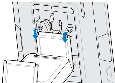
11. Tighten the screws at the top of the KC50 to secure it to the stand.
