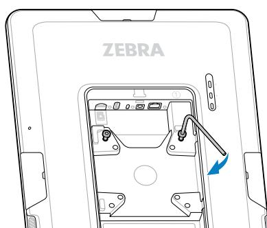
10. Hang the KC50 on the VESA mounting plate by sliding the two screws into the VESA screw slots.
