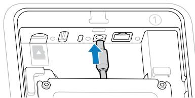
13. Connect the USB-C cable to the USB-C port.
