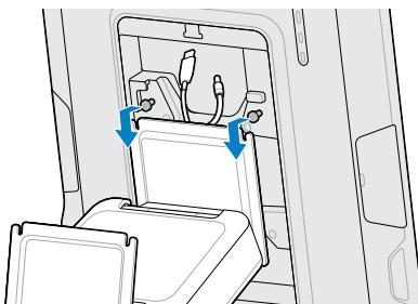
6. Tighten the screws at the top of the TD50 to secure it to the stand.
