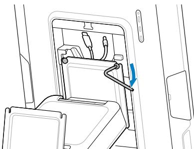
7. Secure the bottom of the TD50 to the VESA plate by attaching the two remaining screws.
