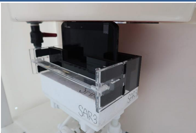
Edge 1 with Battery 1 at 0 mm
