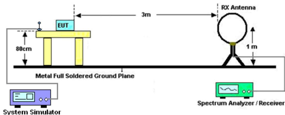
For radiated test from 30MHz to 1GHz
