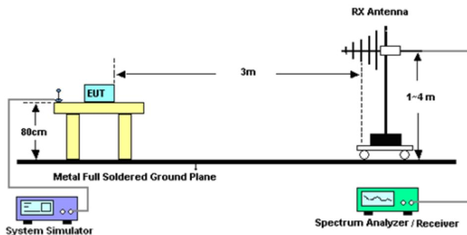
**For radiated test above 1GHz**
