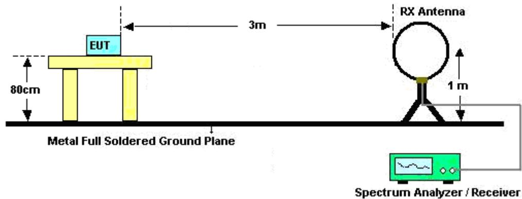
For radiated emissions from 30MHz to 1GHz
