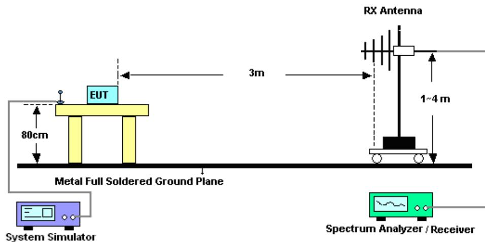
For radiated test above 1GHz
