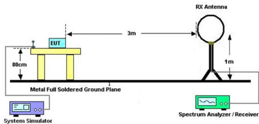
For radiated emissions from 30MHz to 1GHz
