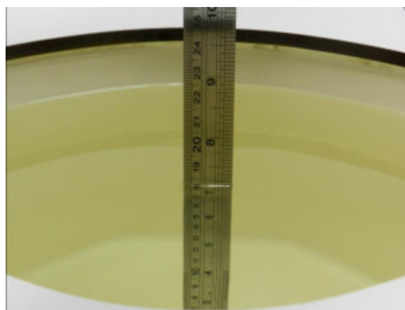
Fig 11.2 Photo of Liquid Height for Body SAR
