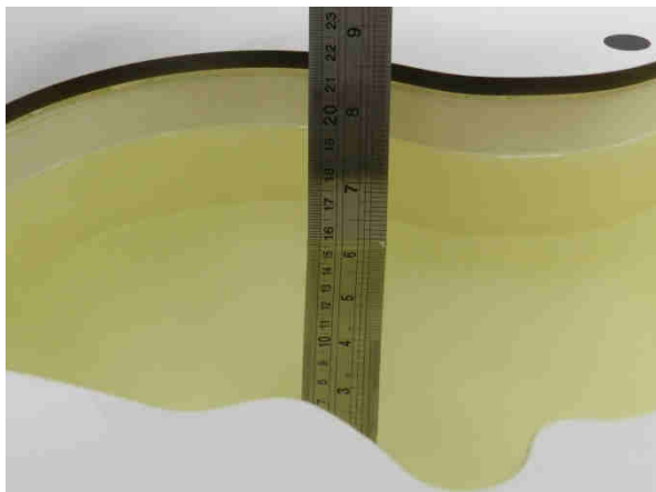
Fig 11.1 Photo of Liquid Height for Head SAR
