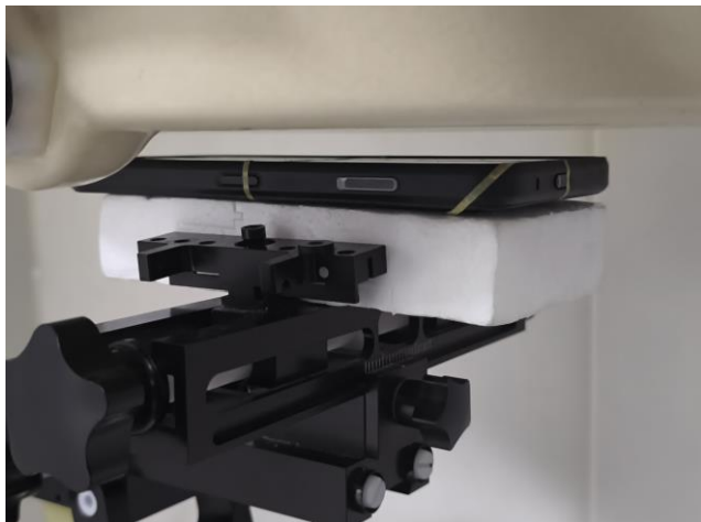
Front, Test Separation 10 mm
