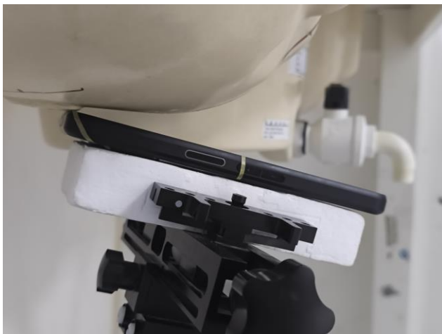
Right Tilted, Test Separation 0 mm
