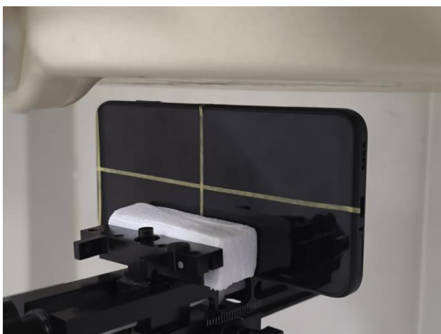
Right Side, Test Separation 10 mm
