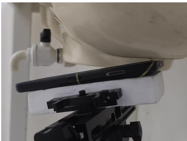
Left Tilted, Test Separation 0 mm
