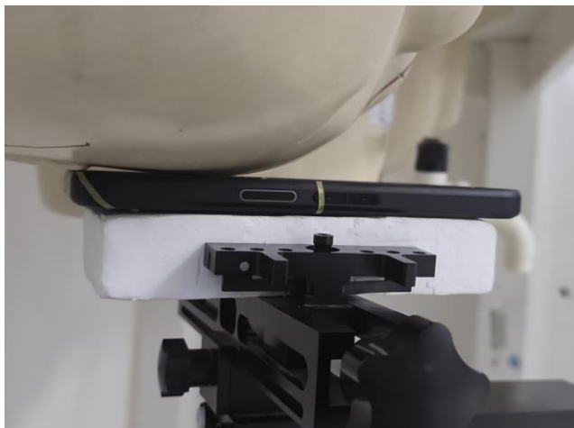
Right Cheek, Test Separation 0 mm
