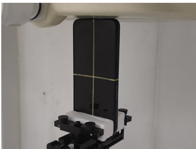
Bottom Side, Test Separation 0 mm
