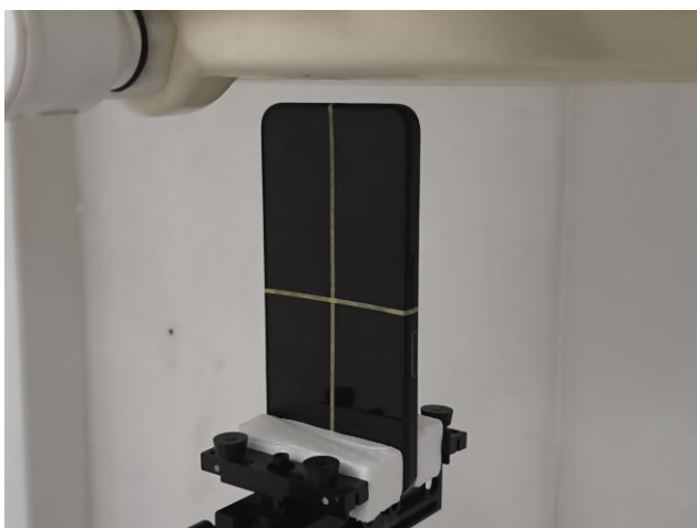
Bottom Side, Test Separation 10 mm
